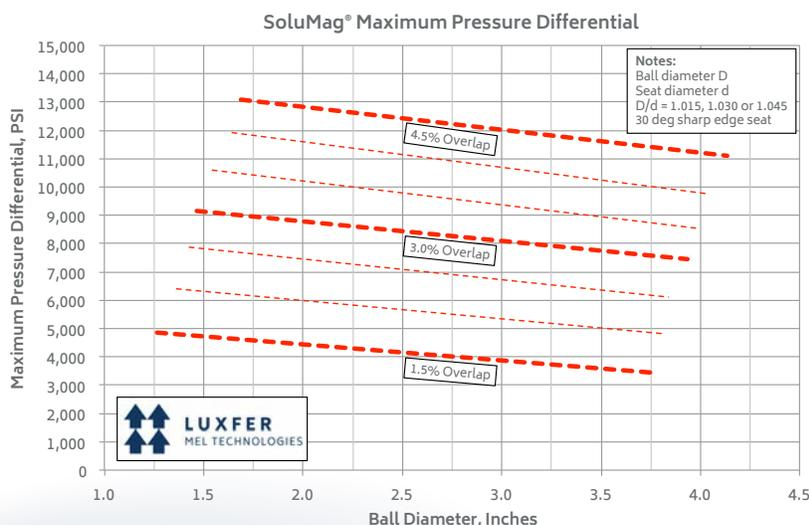
Chart 5. Maximum differential pressure for a SoluMag 1100 ball on a seat.
