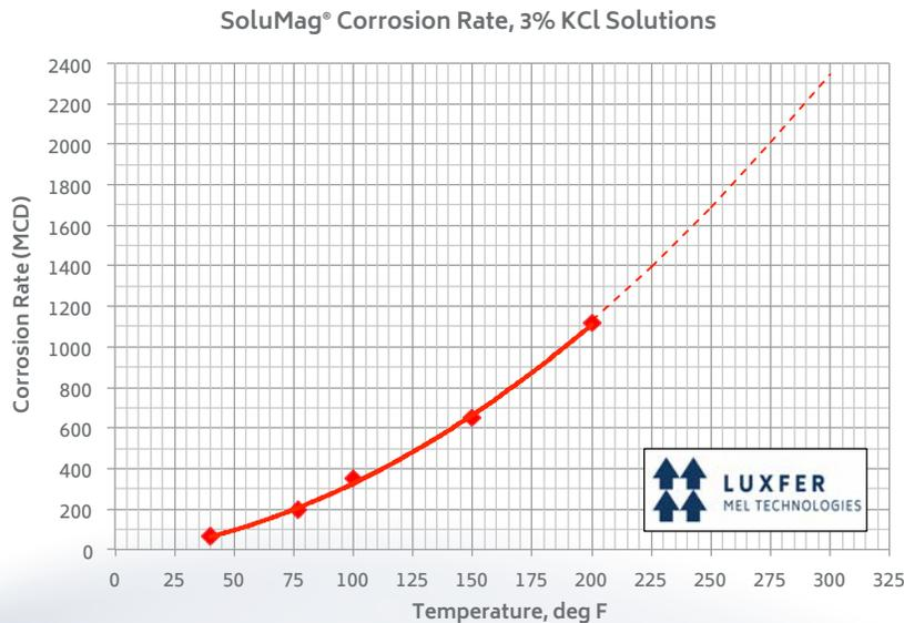
Chart 2. Corrosion rate vs temperature for SoluMag 1100.
