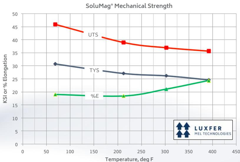
Chart 4. SoluMag 1100 mechanical properties at various temperatures.
