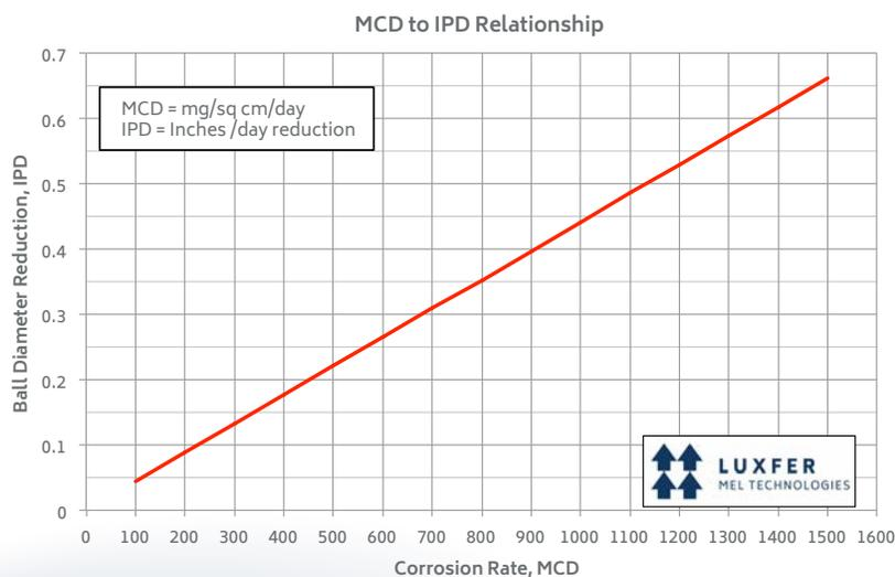
Chart 3. Corrosion rate in relation to inches per day reduction of a ball diameter.
