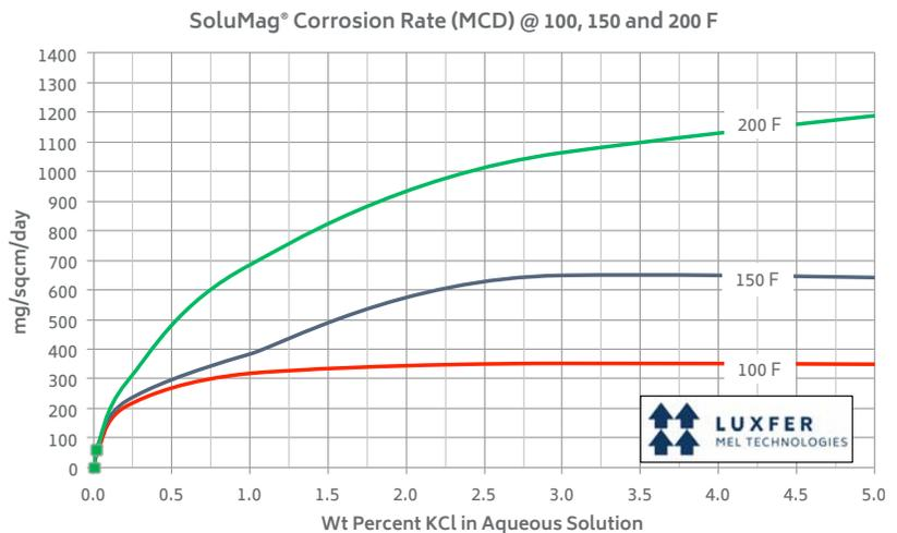
Chart 1. Corrosion rate vs salinity at different temperatures for SoluMag 1100.
