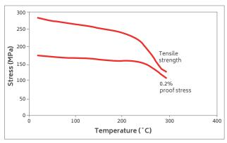
Figure 1. Effect of temperature on tensile properties.
