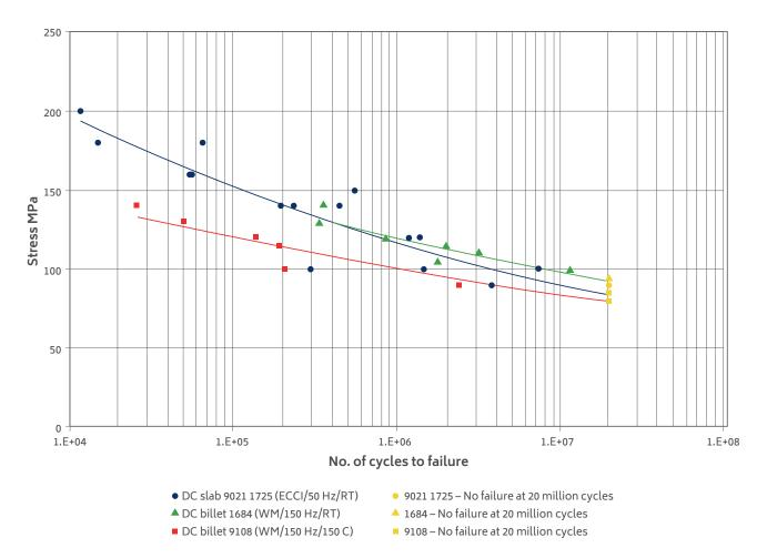
Figure 2. Fatigue curves for DC cast Elektron 21, tested at room and elevated temperature at rotating frequencies 50 Hz and 150 Hz adjusted to a run out of 20 million cycles.
