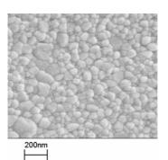
Highly dispersed particles and uniform grain size at sintering temperatures < 1200°C
